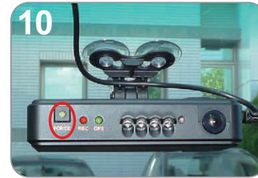
Emergency Button : Light on when power is connected successfully.
