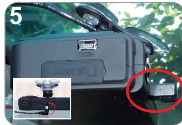
Connect the power cable (plug in either 5 or 6 socket, please do not plug in both sockets at the same time)
