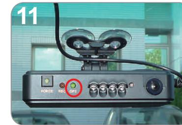
Green : Flashing while GPS is positioning
