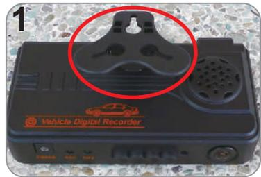
Make the bracket facing upward
