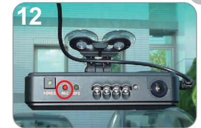
Red : Flashing during recording
