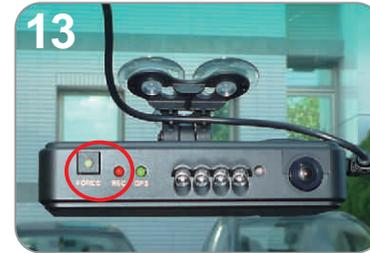
Emergency Button: When press down, the red light will flashing rapidly. In nighttime its LED will light on as indicator.
